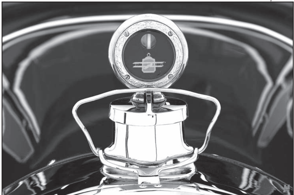
Above: Motometers, designed as practical, utilitarian tools, were integrated into elaborate and distinctive hood ornamentation, and were adapted to different models of automobiles made by the same manufacturer. Below: Although the gauges are similar, the Packard hood ornament above is quite distinct from this Packard Eight 1928 Dual Phaeton mounting.
