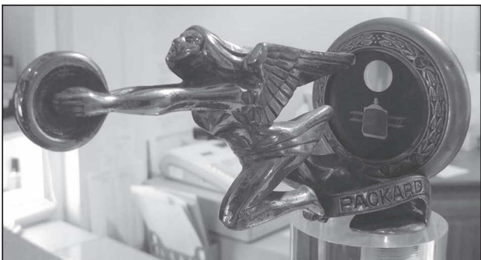
Above: Motometers, designed as practical, utilitarian tools, were integrated into elaborate and distinctive hood ornamentation, and were adapted to different models of automobiles made by the same manufacturer. Below: Although the gauges are similar, the Packard hood ornament above is quite distinct from this Packard Eight 1928 Dual Phaeton mounting.
