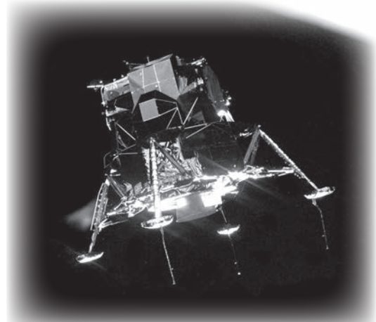
Apollo 11 Lunar Module Eagle in landing configuration in lunar orbit from the Command and Service Module Columbia. NASA
