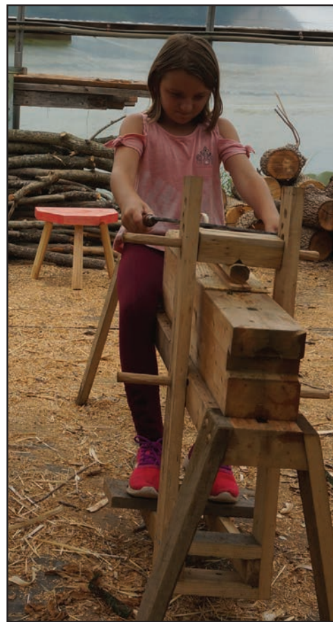
Above: Eden McMillan gives the shavehorse and drawknife a try. Left: Logan Youngman tapers the tenon on a stool leg. The bit brace used to create the mortises and tenons was used by Touris' grandfather.
