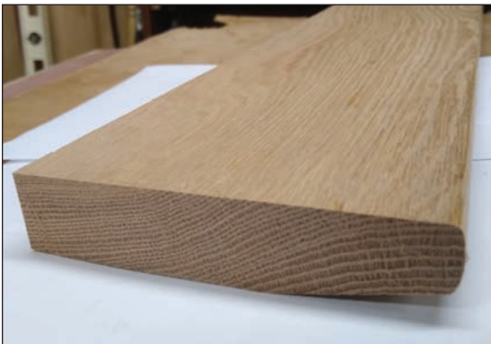
Plain sawn oak: note the growth ring direction and no ray flecks on the face.
