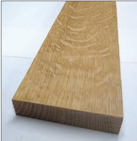
Quartersawn white oak: note the growth rings are almost perpendicular to the board face. Observe the pronounced patterns of the ray flecks.
